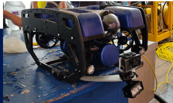
ROV for underwater visual inspections
