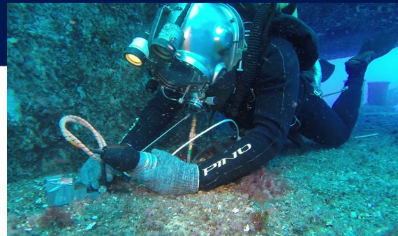
Ultrasound Thickness Measurement
