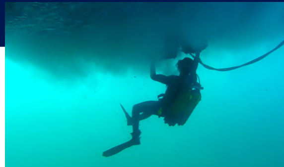
Hull cleaning with hydraulic brushes
