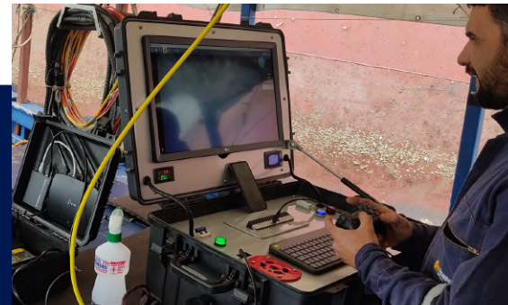
Remote ROV operator system for underwater visual inspection
