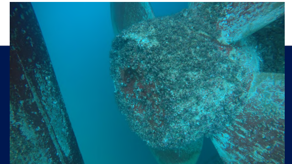
Captured image by ROV, for analysis of the condition of the propeller
