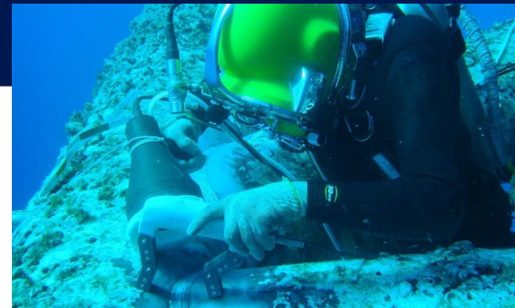
Magnetic Particle Testing
